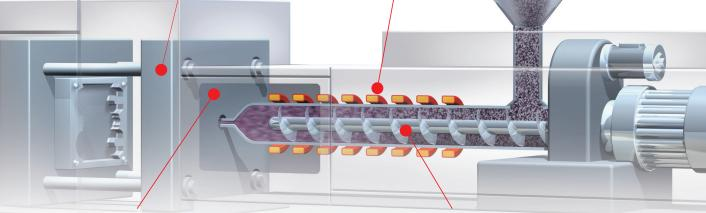
Resin exits nozzle and is injected into mold. During a purge the nozzle is pulled back and resin is pushed out. Once the new resin comes out without any specks or streaking, the molding machine is put back into service. Heater bands cover barrel to melt plastic resin. Resin will bake onto the barrel and bits of old resin will flake off, which will impact quality. Over time resin "bakes on" barrel and screw.
