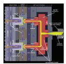
Hot runners heat the resin to the specified flow melt temperature so resin properly fills the mold cavity and leaves no voids. Hot runners need to be cleared of old resin before starting a new molding process.
