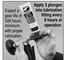
Expect a gear life of 500 hours minimum, with proper lubrication.
